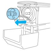
Rotate the handwheel (about 50 degrees) to move the race of the hook to a position where it can easily be oiled.
